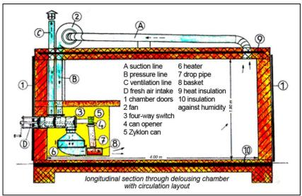
**Fig. 4:** DEGESCH delousing chamber with circulation feature. <sup>52</sup> This design was developed in the late 1930s / early 1940s and became a standard in Germany during the war. It was, however, not installed in all concentration camps, which were frequently equipped with makeshift delousing chambers. Editor's note.
