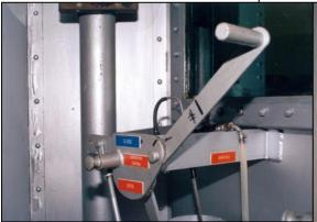
**Fig. 100 (top):** Lever used to release gas pellets into chemical solution.
