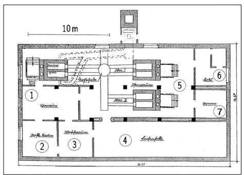
Fig. 5: Ground plan of Crematorium I in Auschwitz I/Main Camp in its original condition. The morgue was later allegedly used as a homicidal gas chamber. 1: vestibule; 2: laying-out room; 3: wash room; 4: morgue; 5: furnace room; 6: coke; 7: urns
