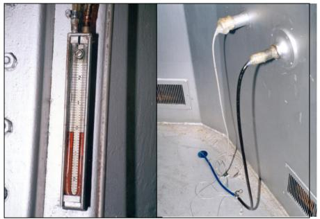
**Fig. 110:** Manometer to monitor relative gas chamber pressure.
